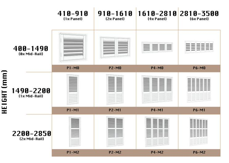
If a Mid Rail is required it will be placed at 600mm from the base.
